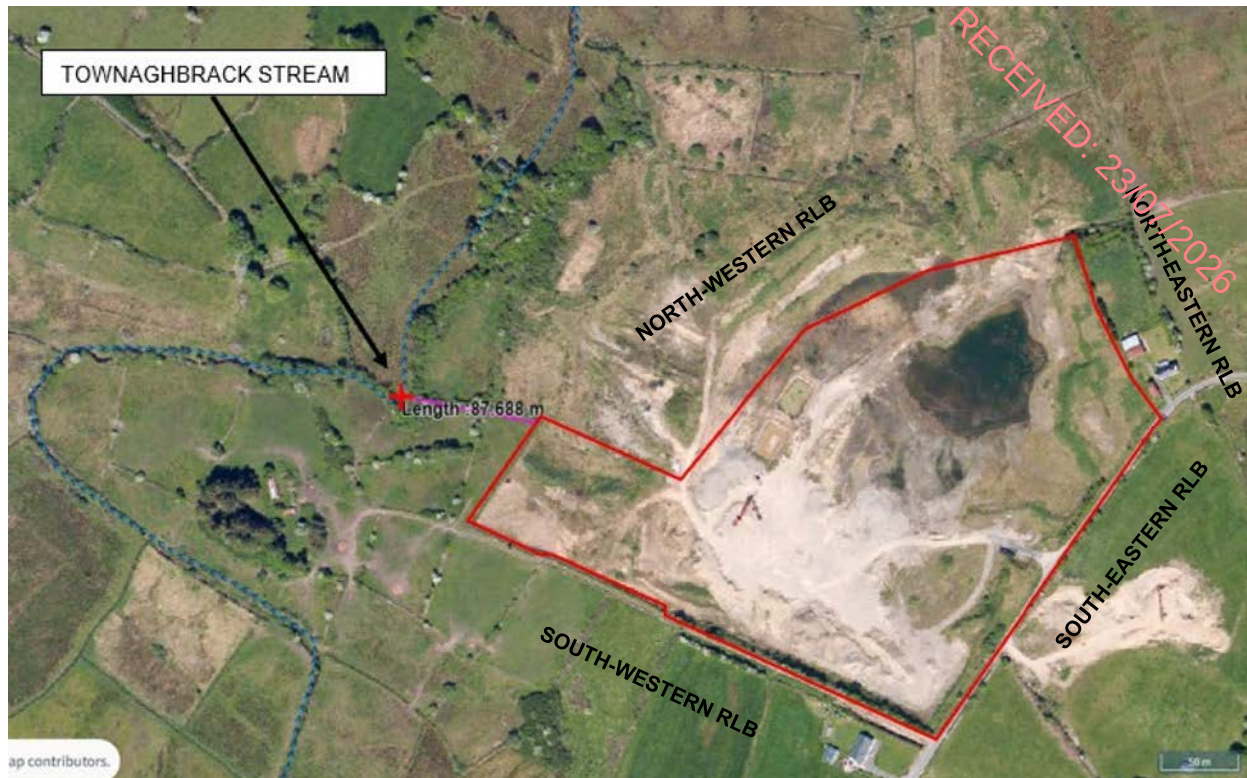
Figure 3.1 Proposed site location (red) in relation to the Townaghbrack stream that has potential connectivity to the Templehouse and Clooncleigha Loughs SAC and Unshin River SAC downstream towards the north of the site via the existing drainage network associated with the former extraction area (image shown Figure 2.10).
